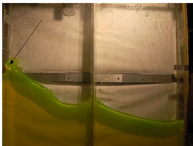
FIG. 16. (Color online) Formation of a gas pocket at the vertical walls occurring for \eta_{2a}/l = 0.03 and h/l = 0.35 . The photograph and video is given for \sigma/\sigma_1 = 0.96 and Sn = 0.472\,857 (enhanced online). [URL: http://dx.doi.org/10.1063/1.3562310.6 ]
