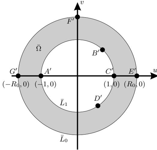
Fig. 2.1. Cross section in mapped two long eccentric cylinders with parallel axis.
