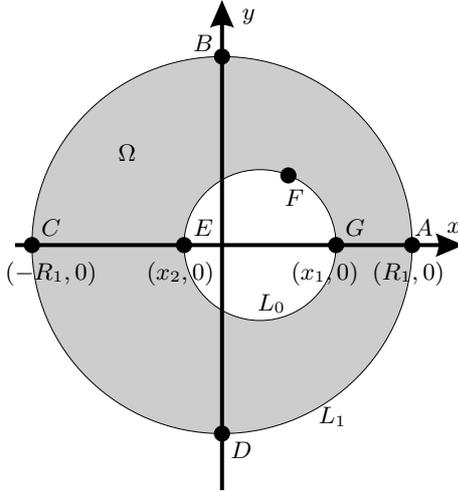
Fig. 1.1. Cross section in two long eccentric cylinders with parallel axis where  $-R_1 < x_2 < x_1 < R_1$ .
