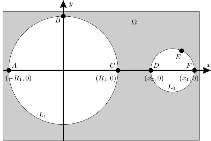
Fig. 1.2. Cross section in two long parallel cylinders where  $R_1 < x_2 < x_1$ .
