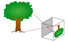
Figure 1. A pinhole camera, http://en.wikipedia.org/wiki/File:Pinhole-camera.png.
