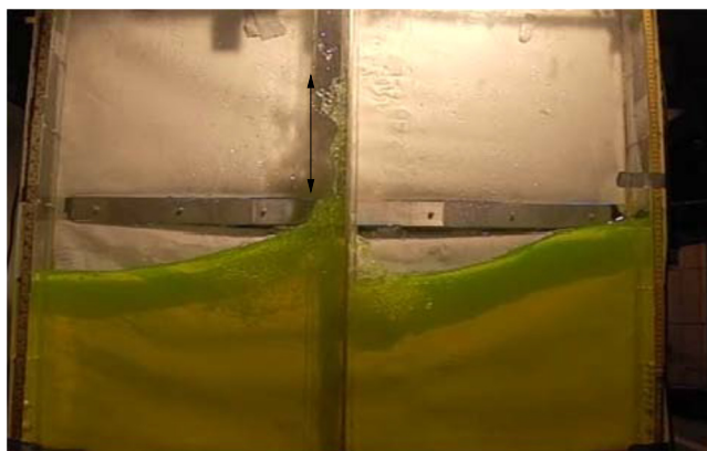
FIG. 12. (Color online) The photograph and video recording of the runup at the screen occurring for 0.9 \leq Sn (enhanced online). [URL: http://dx.doi.org/10.1063/1.3562310.4 ]
